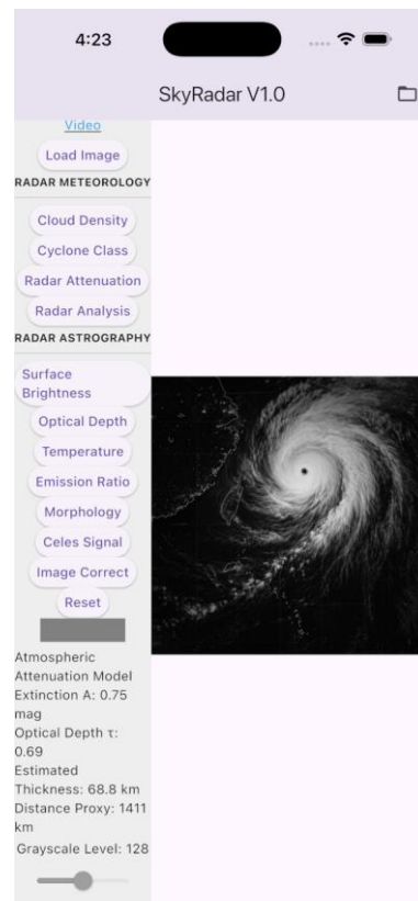
Fig. 5 Radar Attenuation map produced by SkyRadar, displaying extinction (mag), optical depth ( \tau ), and estimated atmospheric thickness. Higher extinction values indicate strong radar beam attenuation through dense clouds or precipitation
